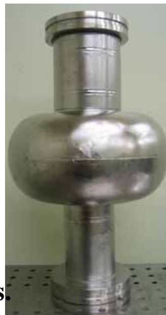
LL End single cell cavity (End cell shape)
