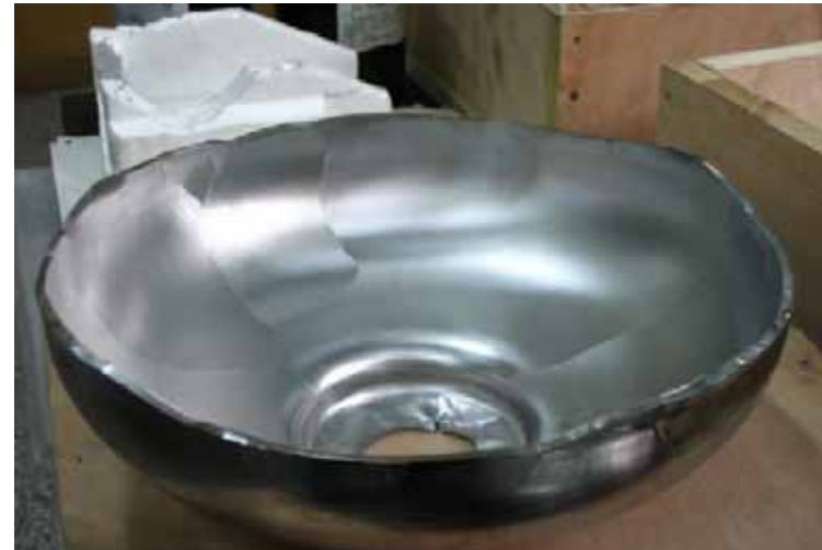
PKU Large Grain cavity after post-purification at 1250C
