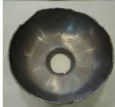
Directly formed the sliced sheets. No annealed the sheets.
